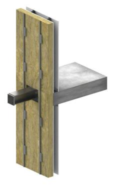
Figure 2: Detail 1, Sapphire G60/G25 through an exterior insulated steel famed wall
